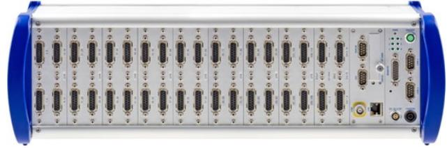
*The measurement system provides CAN FD connectivity (Photo: IMC)*
