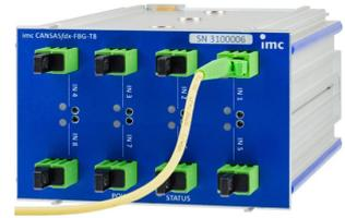
*A variety of measurement, testing, and control applications can be covered, and a range of vehicle and industrial buses such as CAN can be integrated (Photo: IMC)*
