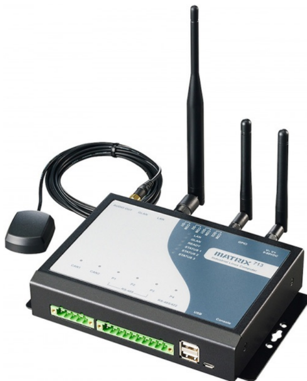
Besides CAN, isolated EIA-485 serial ports, digital I/O, and Ethernet ports are available (Photo: Artila)
