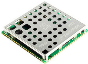
The IPC@Chip embedded controller features two CAN ports (Photo: HMS)
