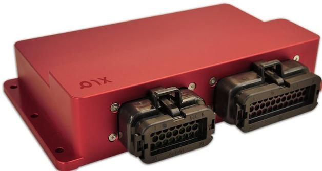
The IP67-rated control units come with CAN interfaces (Photo: Pix)
