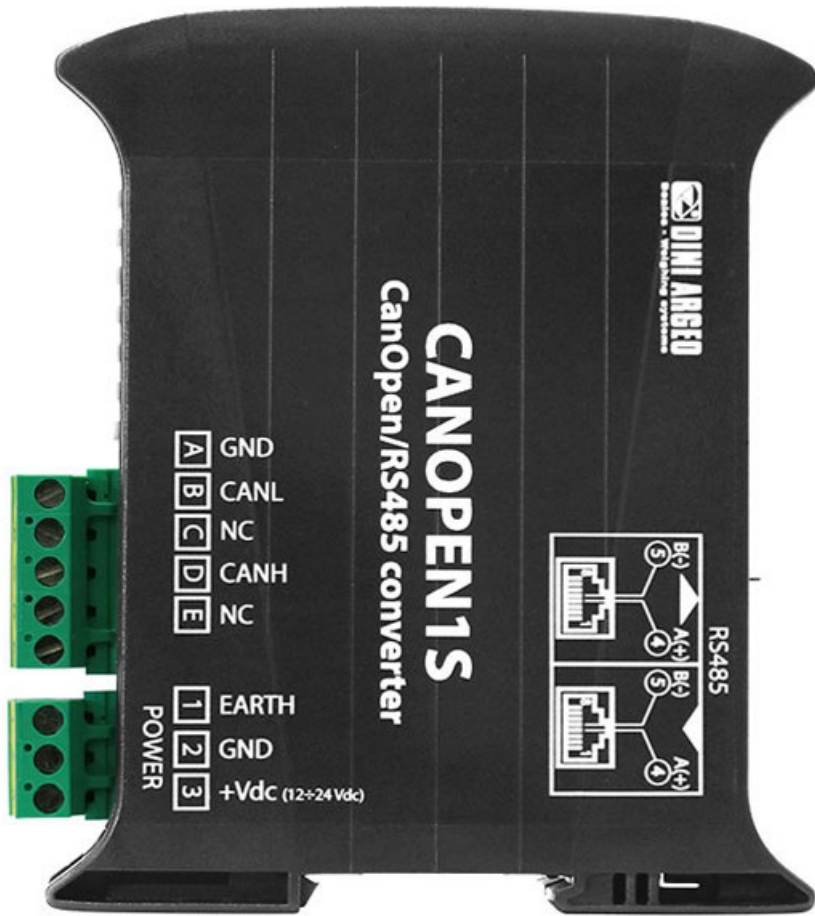
CANopen interface unit with calibration and configuration capabilities (Photo: Dini Argeo) Zoom
