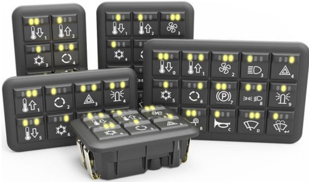
The keypads are IP67-rated and vibration and impact resistant (Photo: Grayhill)
