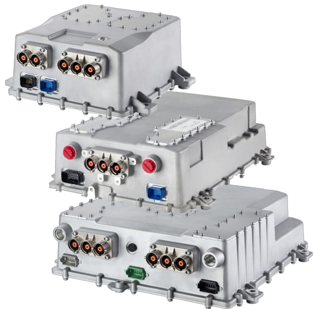
The WTI traction controller features CAN connectivity (Photo: Curtiss-Wright)
