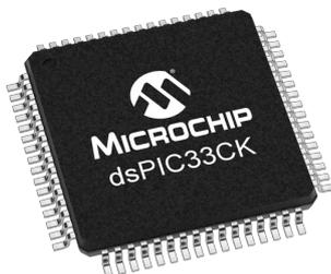
The 16-bit digital signal processor comes in eight packaging variants with 28 to 80 pins measuring 5 mm x 5 mm (Photo: Microchip)
