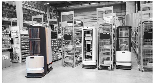
The Toru logistics robot combines autonomous driving with handling robotics (Photo: Magazino)
