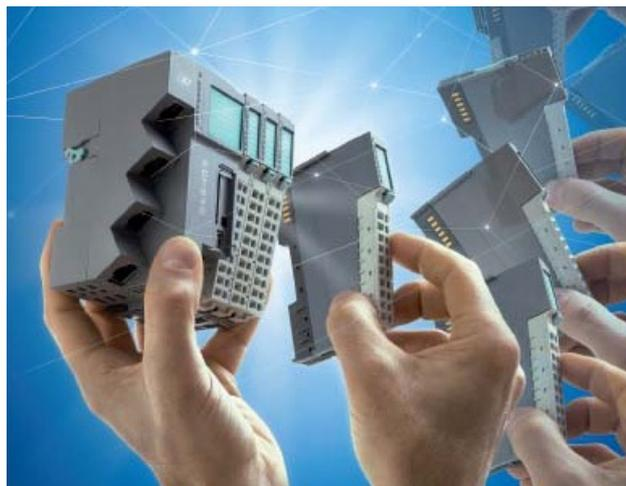
The FCT640 modular host controller can feature up to 1024 local digital I/O ports or up to 512 analog I/O channels (Photo: CMZ)
