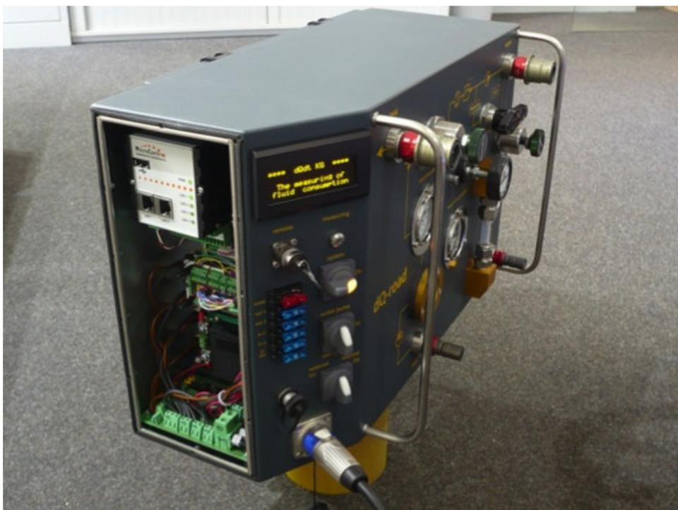
In the robust casing of the dQ-road, Roland Czech has placed the entire measurement and CAN technology which is controlled by the Linux control unit  $\mu$ MIC.200 (Photo: dQdt)
