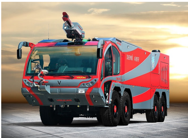
The front-axle is steered mechanically, while the rear-axle uses an electrohydraulic steering (Photo: Volkan)
