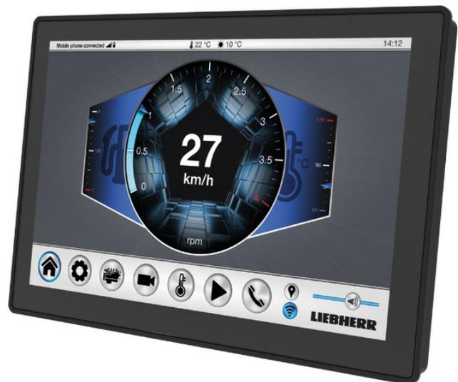
DC5 can be used as control computer, display, or input device (Photo: Liebherr)
