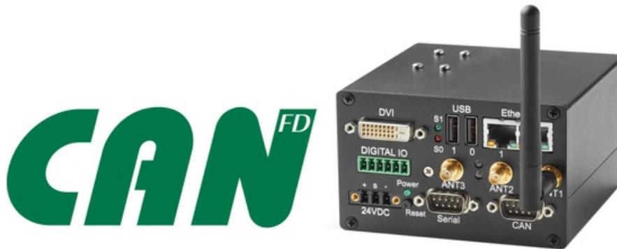
In comparison to Classical CAN networks, CAN FD networks offer a higher bandwidth and are highly robust (Photo: Janz Tec)
