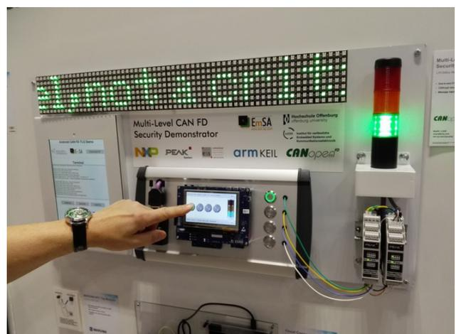
CANcrypt combined with the secure transceiver by NXP enables cyber security in open network approaches (Photo: Emsa)
