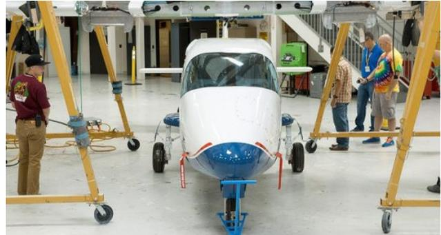
*Technicians at Scaled Composites in Mojave (CA) install a wing designed for electric motors onto a Tecnam P2006T to form the X-57 Maxwell battery-powered plane (Photo: NASA)*
