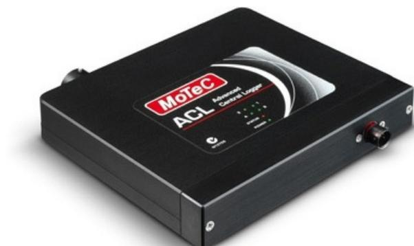
*The ACL logger communicates via CAN with multiple SVIM input modules (Photo: Motec)*
