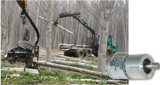
Speed and length measurement directly in the tool (Photo: Wachendorff)
