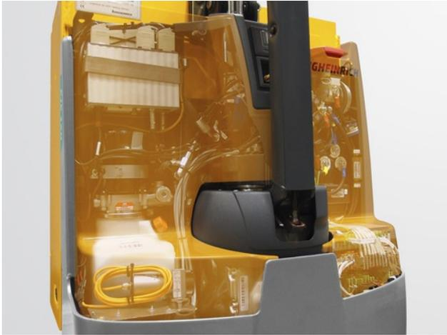
Data recorder and universal amplifier in the EJE series of electric walkie pallet trucks (Photo: HBM/Jungheinrich)
