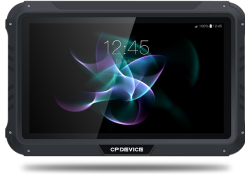
The Apollo 10 comprises a 10,1-inch touch-screen (Photo: CP Device)
