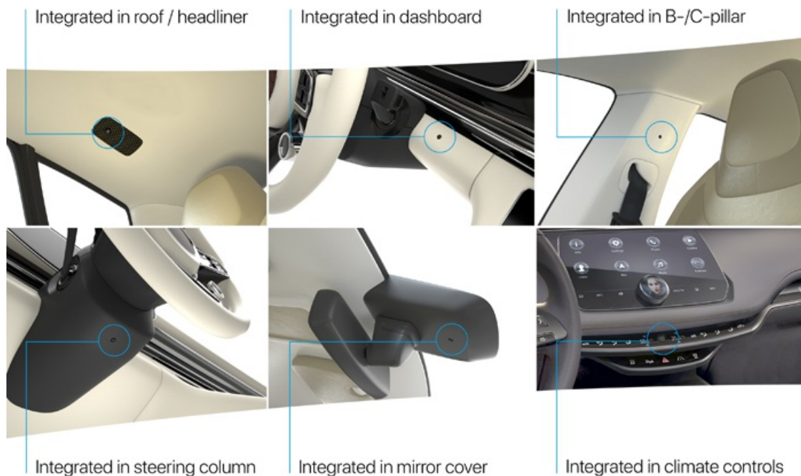
CAN-linked temperature sensors can be placed far away from the air-conditioning ECU (Photo: Preh)
