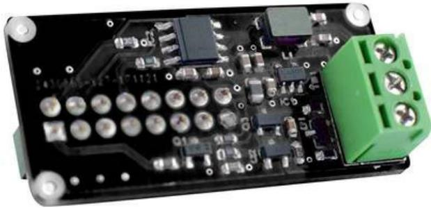
*The CAN interface module is intended for the SGD 70-A capacitive touch display (Photo: Lascar Electronics)*
