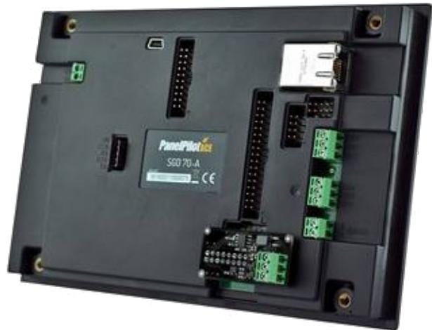
*The backside of the SGD 70-A display with mounted S-70-CAN module (Photo: Lascar Electronics)*
