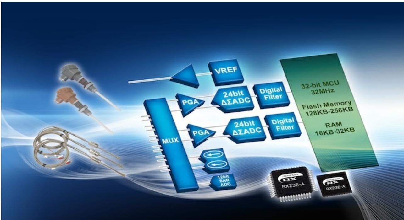
The RX23E-A combines an analog front-end with a 32-bit micro-controller providing an on-chip CAN controller (Photo: Renesas)
