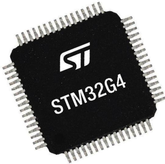
*The STM32G4 Series combines a 32-bit Arm Cortex-M4 core (with FPU and DSP instructions) with 3 different hardware accelerators: ART Accelerator, CCM-SRAM routine booster, and mathematical accelerators (Photo: STMicroelectronics)*
