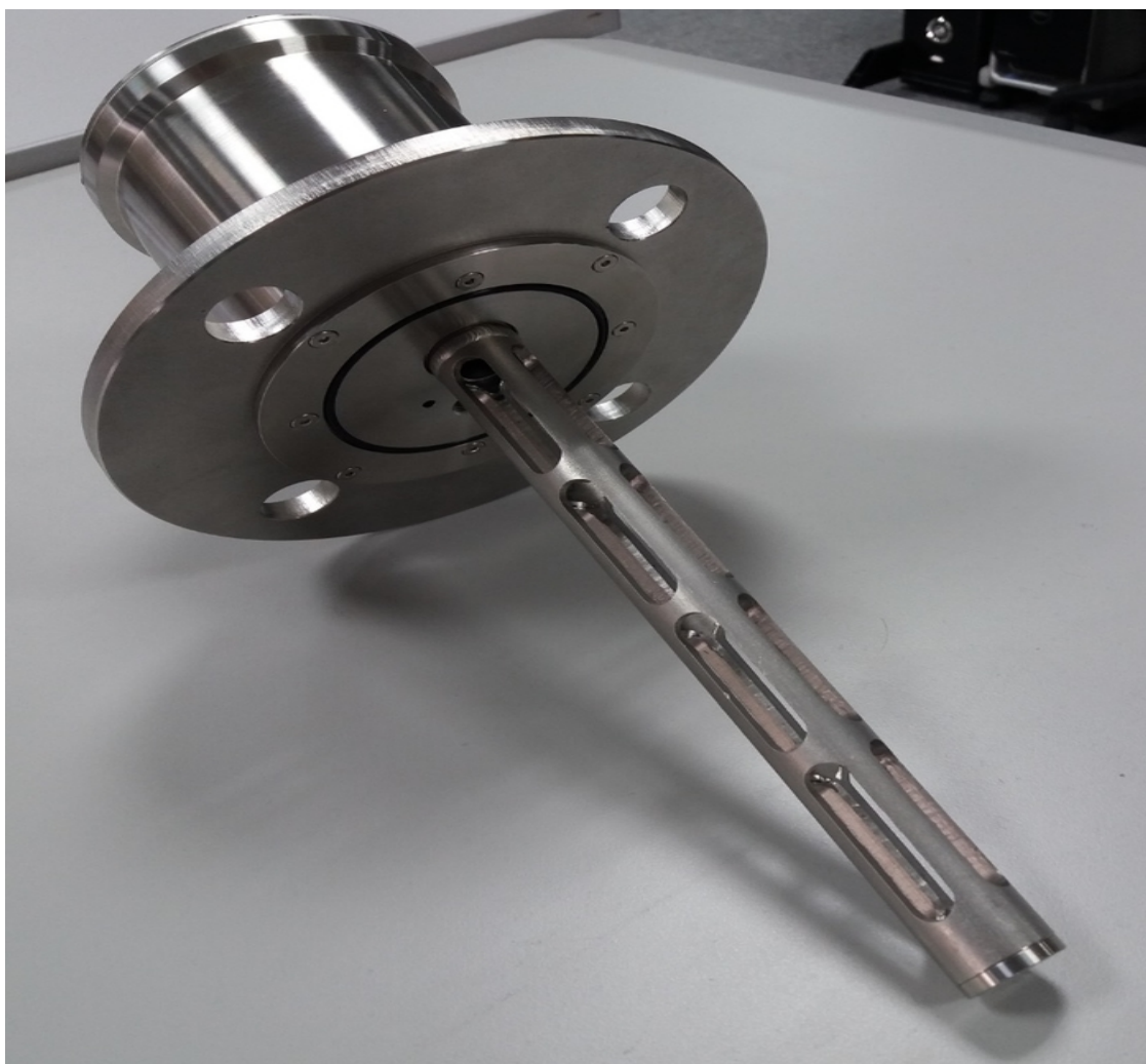
CMR shows its Niris (near infrared intelligent sensor) natural gas sensor at Cimac 2019 (Photo: CMR)
