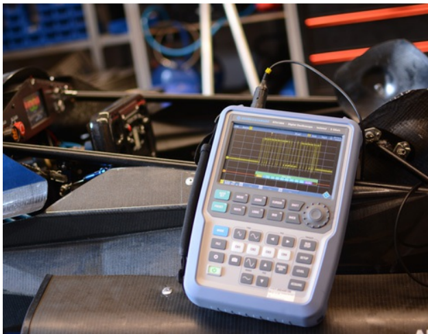
Debugging CAN data (Source: FaSTDa Racing Team)
