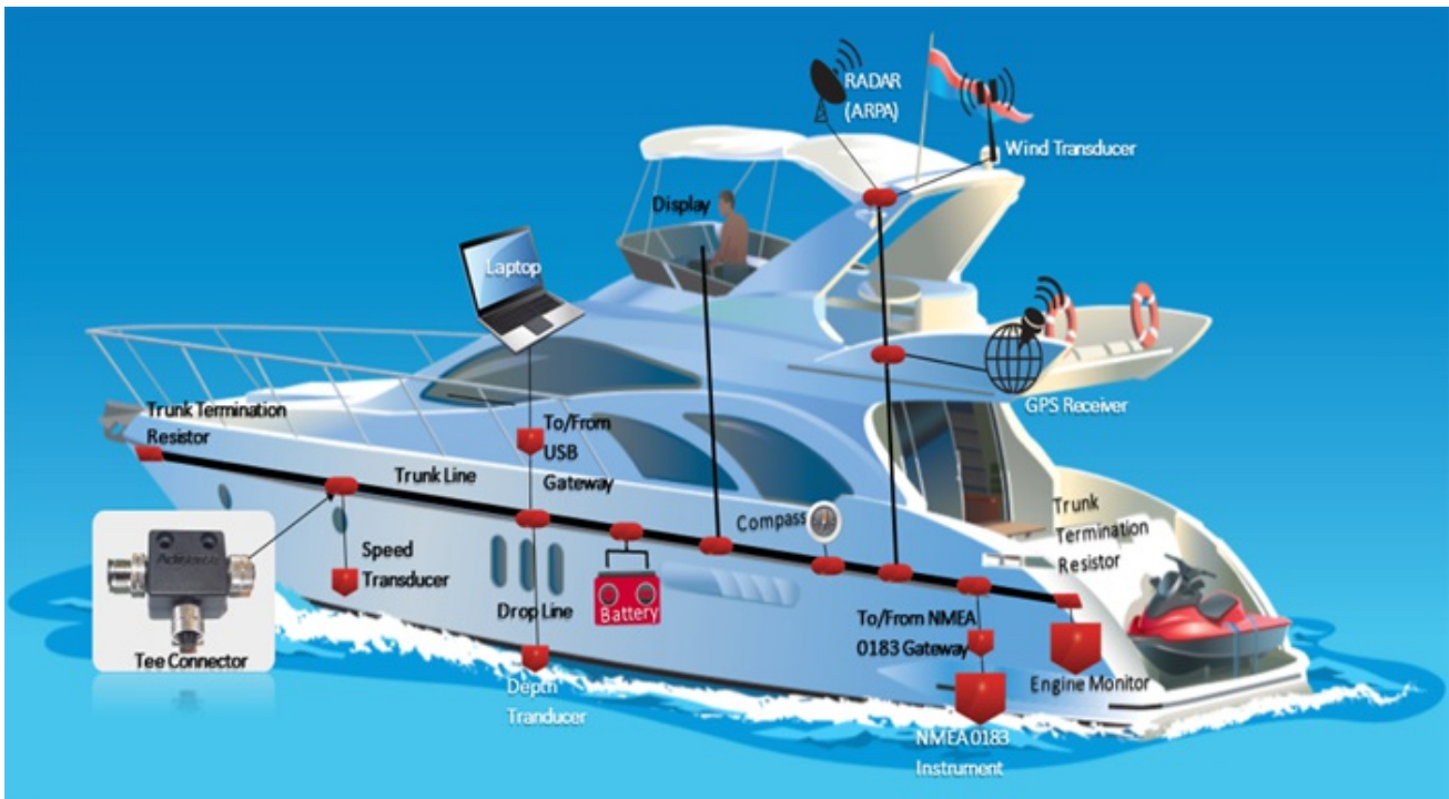
The J1939-based NMEA 2000 application profile is standardized in IEC 61162-3 (Source: Warwick Control Technologies)
