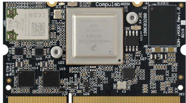
The SoM is intended for human machine interface devices in different application fields including industrial automation and medical devices (Source: Compulab)
