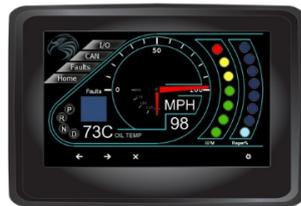
The VeeCAN 800 unit is completely sealed to IP66 (front) and IP67 (back) making it electronically and environmentally rugged to meet the challenges of providing instrumentation for harsh environments (Source: New Eagle)
