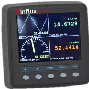
The Influx Technologies Rebel Dash; With a straightforward mounting system, there can be monitored vehicle CAN data graphically within minutes (Source: Influx Technologies)
