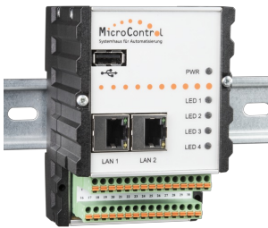
The CANopen controllers are programmable in Node-RED and C/C++ (Source: Microcontrol)
