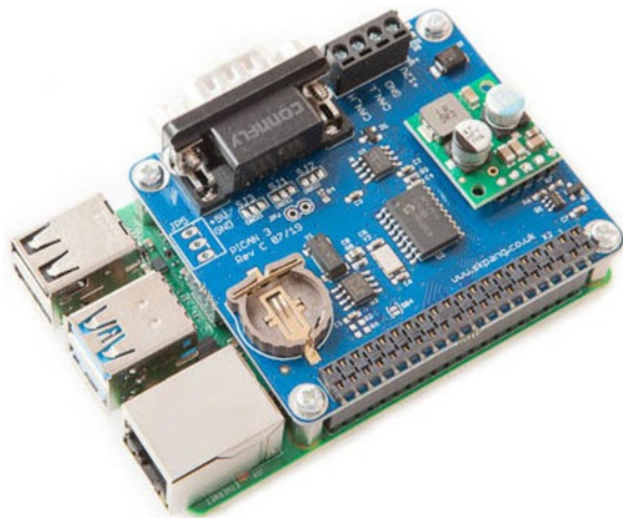
The PiCAN3 is equipped with a CAN transceiver and a stand-alone CAN controller by Microchip (Source: Copperhill)
