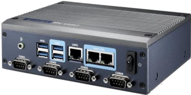
*The embedded system supports multiple storage, which includes onboard eMMC up to 128 GiB, mSATA, and 2.5-inch SSD/HDD for storage options (Source: Advantech)*
