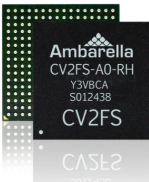
The low-power SoCs include an OTP (one-time-programming) memory for secure booting (Source: Ambarella)
