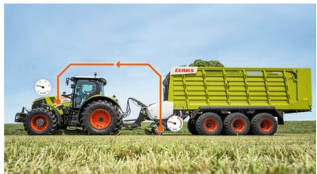
With TIM Speed Control the Cargo 9000 and Cargo 8000 loader wagons are able to control the speed of a tractor (Source: Claas)
