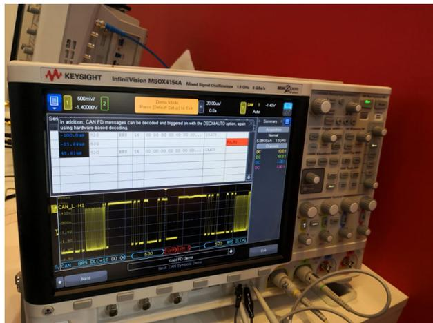
*The CAN FD oscilloscope from Keysight in action (Source: CAN in Automation)*
