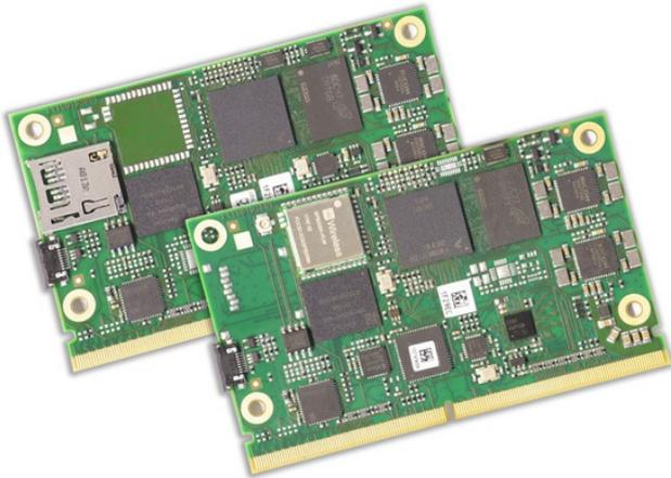
*The series integrates up to four ARM Cortex-A53 processors with up to 1.8 GHz, the ARM Cortex-M4 real time processor, and the Vivante GC Nano Ultra multimedia 2D/3D graphics processor (Source: Avnet Integrated)*
