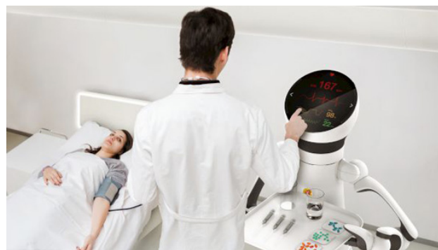
The Care-O-Bot4 service robot can also be used in hospitals; it comprises embedded CAN networks for different purposes (Source: IPA-Fraunhofer)
