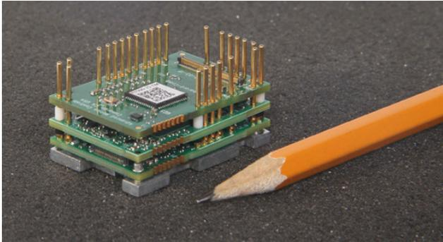
*The products come with torque, velocity, and position operating modes (Source: Advanced Motion Controls)*
