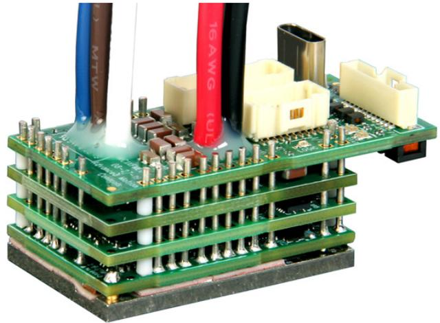
*The servo drives are designed to withstand extreme temperatures, high and low pressures, shocks, vibrations, humidity, dust, dirt, and contamination (Source: Advanced Motion Controls)*
