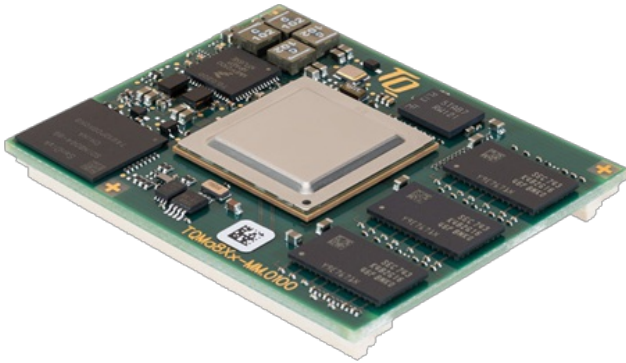
The TQMa8xx module is based on the processor ARM Cortex-A35 core technology (Source: TQ-Systems)
