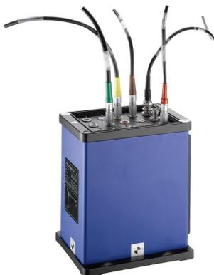
GNSS-aided inertial system with an output rate of 1000 Hz and data latency (Source: Genesys)
