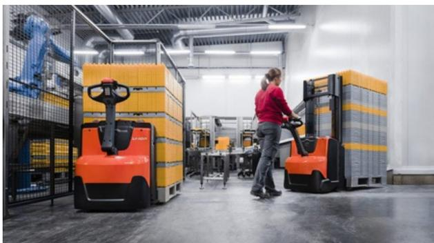
Pedestrian stackers use CAN networks to improve diagnostics and to simplify maintenance; they also reduce the wiring effort (Source: Still)
