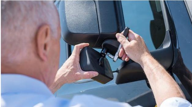
The radar is installed on the right mirror (Source: Continental)
