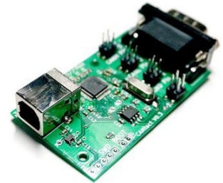
The predecessor CANtact features one CAN interface and a 12-Mbit/s USB interface (Source: Linklayer Labs)
