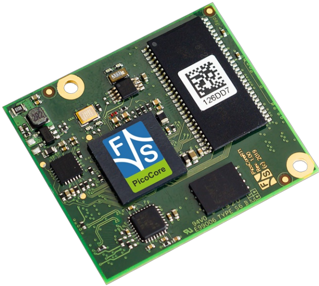
PicoCore RT1 computer-on-module weighs 10 g (Source: F&S)
