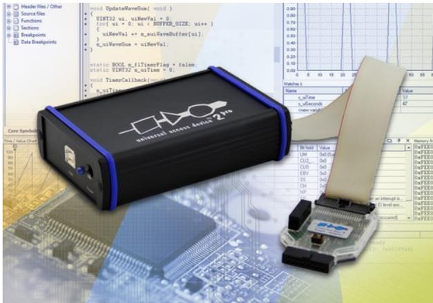
The latest version of the UDE (Universal Debug Engine) supports the S32S247 and i.MX RT MCUs (micro-controller units) (Source: PLS)
