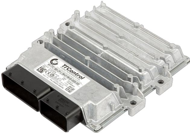
*The ECUs are designed to build up a centralized electronic architecture using one controller for the whole vehicle (Source: TTControl)*
