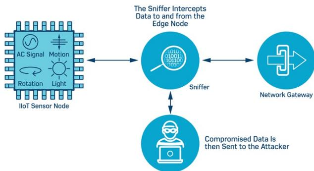
A Man-in-the-middle attack inserts a malicious access point between a node and a gateway (Source: Analog Devices)
