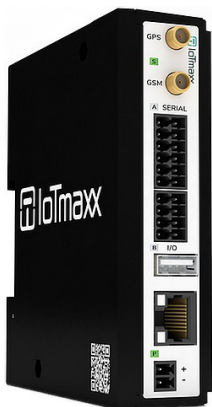
Maxx GW 4100 4-G mobile radio gateway with two integrated SIM card slots (Source: lotmaxx)
