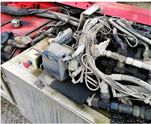
Typical operation environment for an ECU (Source: Epec)
