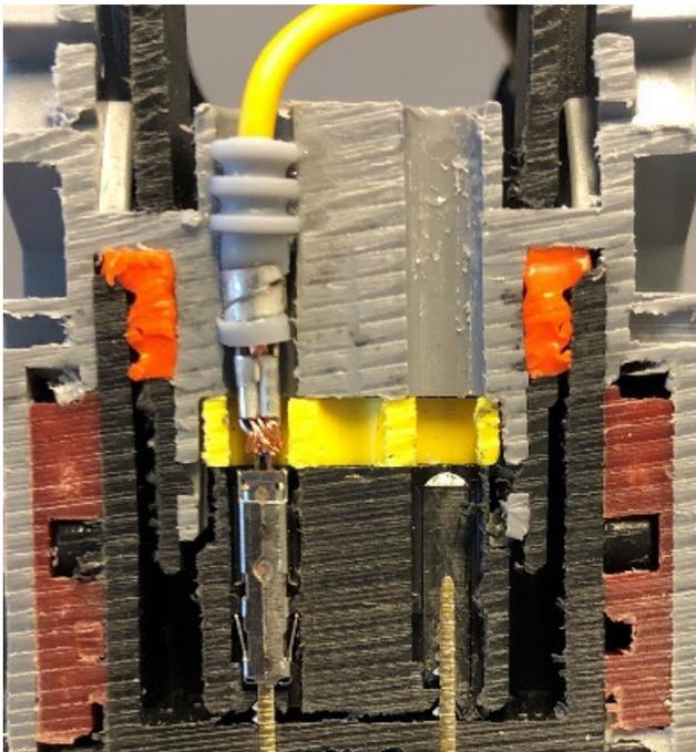
Single wire sealing (SWS) example featuring TE Connectivity's Leavyseal connector (Source: Epec)
