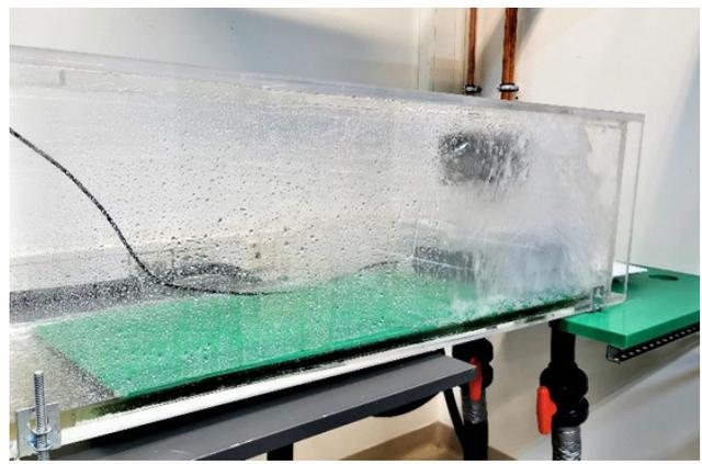
IP65 test performed inside acrylic tube (Source: Epec)
