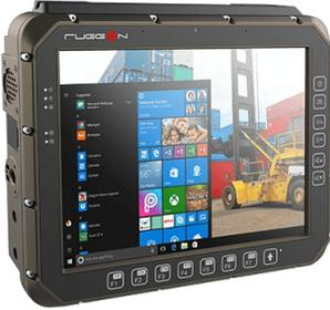
*The auto-dimming touch-screen automatically adjusts visibility for day or night, in-door and out-door (Source: Ruggon)*
